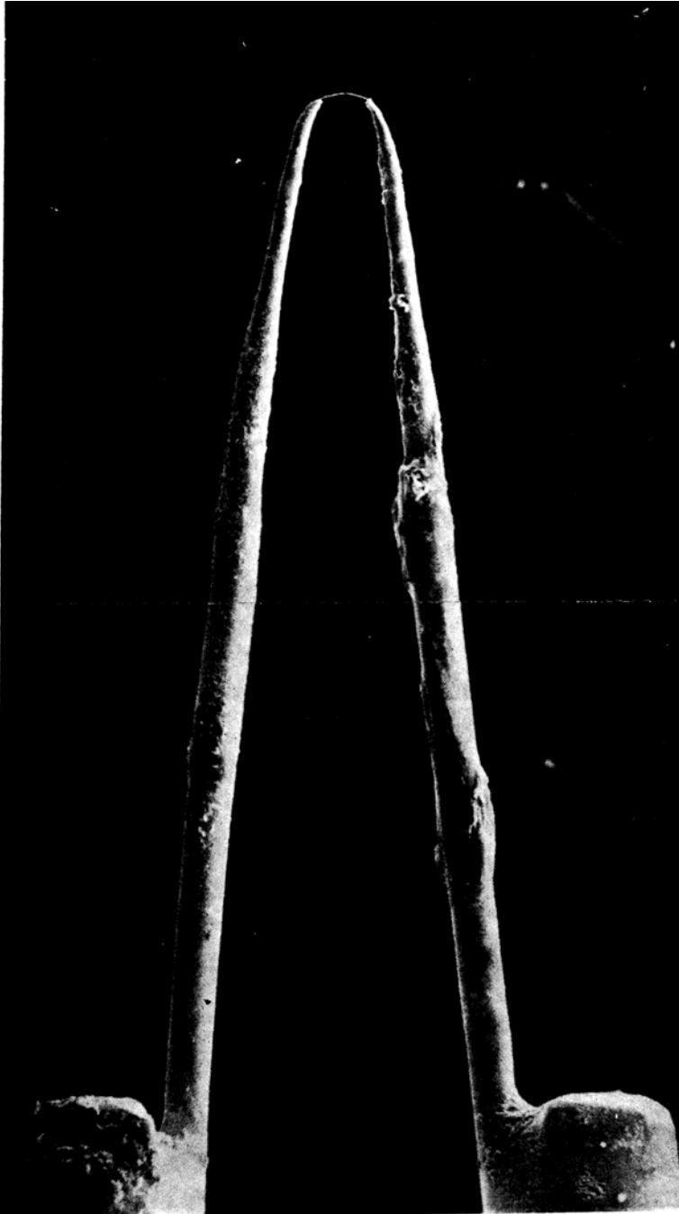
FIGURE 4. Scanning electron microscope photograph of a typical hot wire used in the investigation; length of active element = 100\ \mu\text{m} , diameter of active element = 0.5\ \mu\text{m} .
